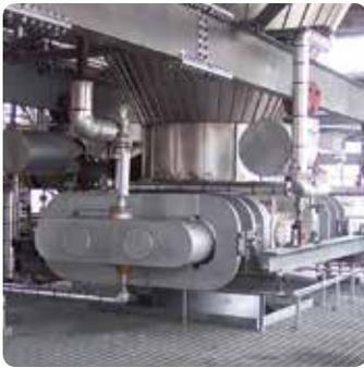
DeltaValve's bottom unheading valves are the lightest, most compact, fully automated unheading valves in the industry. The small footprint of this bottom unheading valve makes it ideal for both space constrained retrofit installations as well as new construction.
