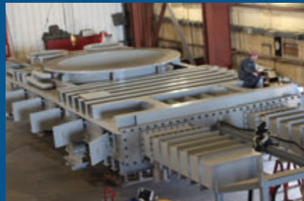
Flue Gas Isolation
