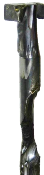
Stem, Disc and Seating Plate Damage Due to Excessive Purging
