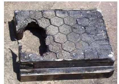
Stem, Disc and Seating Plate Damage Due to Excessive Purging
