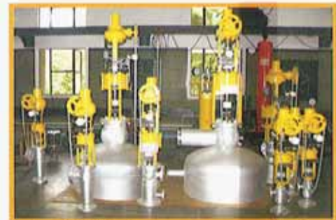
Battery of Turbine bypass, steam conditioning and spray water control valves ready for shipment to Taiwan.
