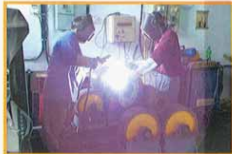
Ongoing welding on forged body
