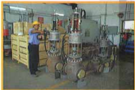
QC NRV undergoing testing
