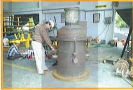
Dump tube ready for inspection
